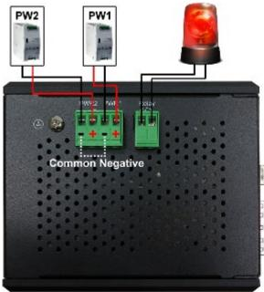
The power inputs are designed as a "common negative", which implies that the negative input is connected, but "double-secure" is supported to prevent the un-notified failure of power from one of the negative inputs. If one of the negative power input fails, the system will detect it and the system will trigger the event if the users set the fault alarm or event log for powers.
